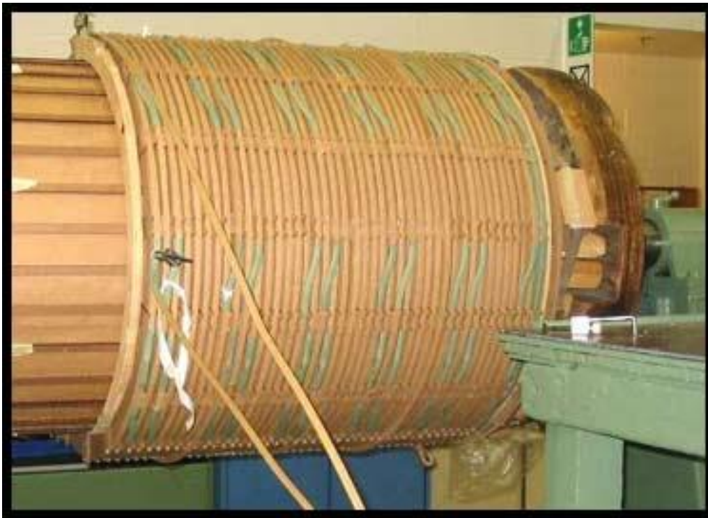
Winding stack under construction
