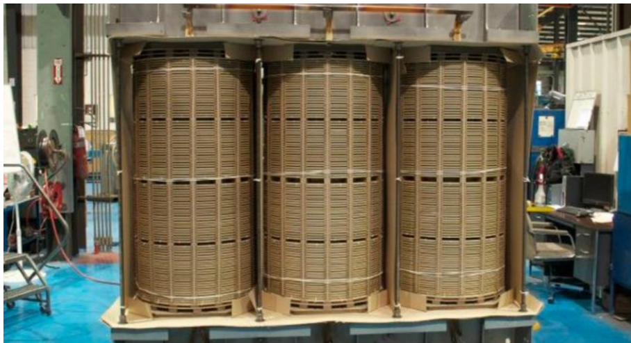
Three-Phase winding assembled with the final core
