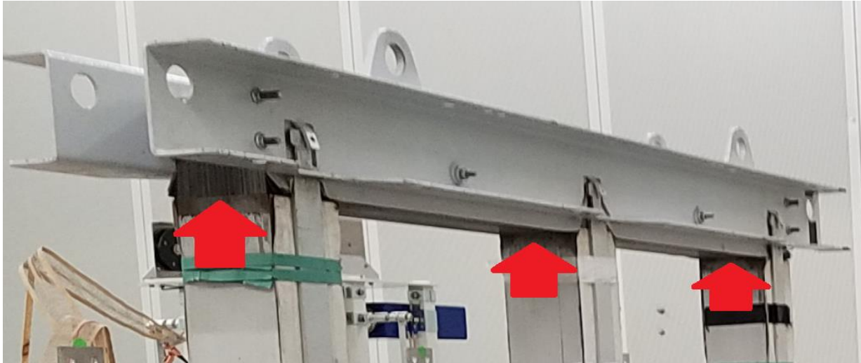
Universal test core with a “butt” joint
